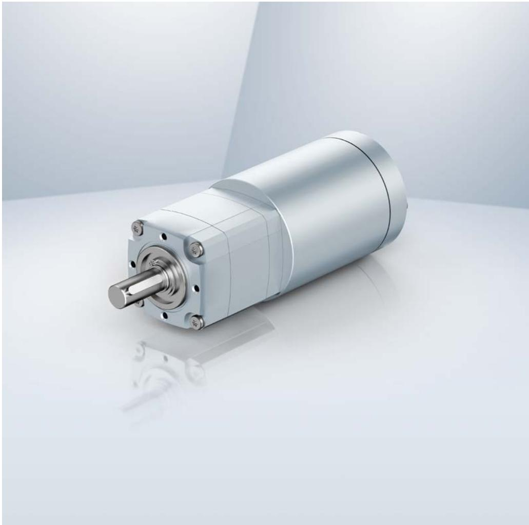
With the installation edge dimensions from 63 mm and a length of just 102 mm in its two-stage design, it offers peak torques of up to 150 Nm.
