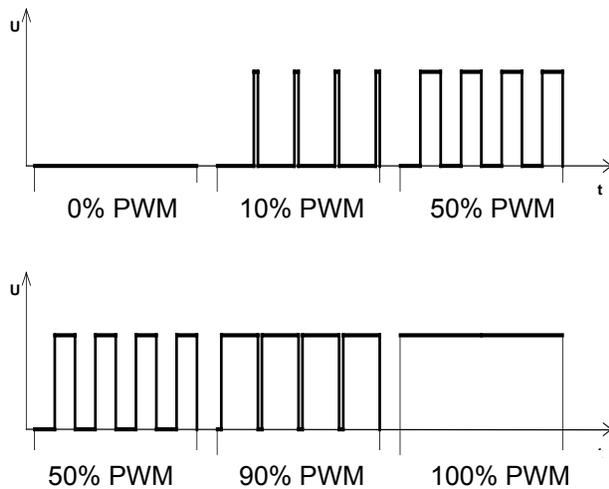
Pulse Width Modulation Signal
