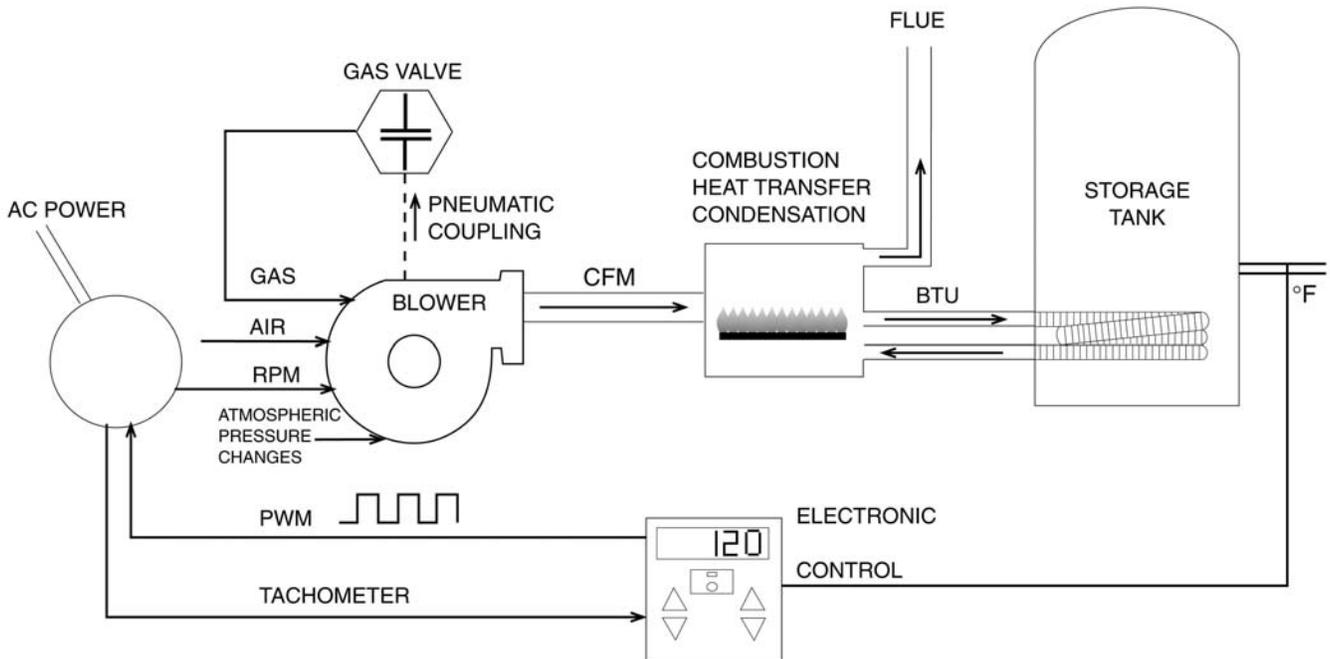
Control logic for a Boiler Combustion System
