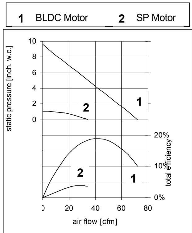
Pressure and Efficiency vs. Air Flow
