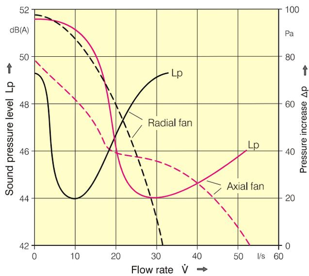
Fig 3: At a glance: acoustic characteristic curves demonstrate noise behaviour during operation.
