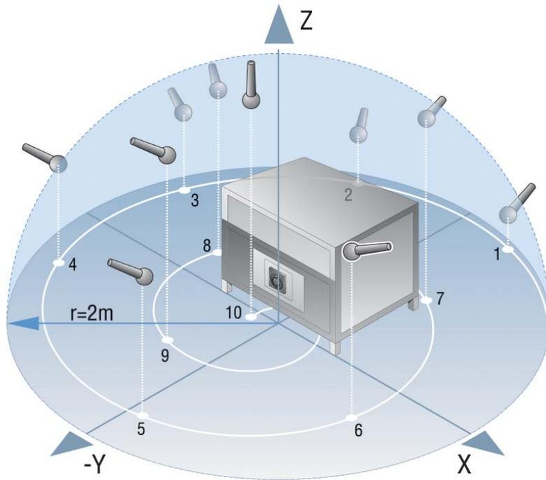
Fig 1: Construction schematic for measuring the acoustic power level
