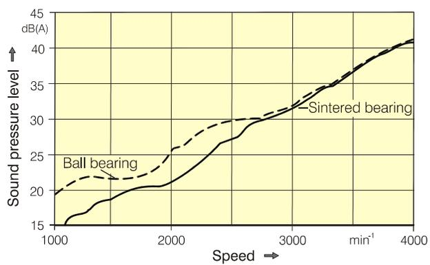
Fig 5: Bearing noise and total sound pressure level
