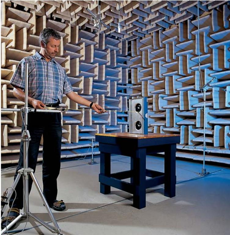
Fig 2: Taking measurements in the anechoic room
