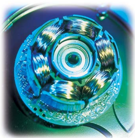
Fig. 4: Programmable fan with integrated microprocessor
