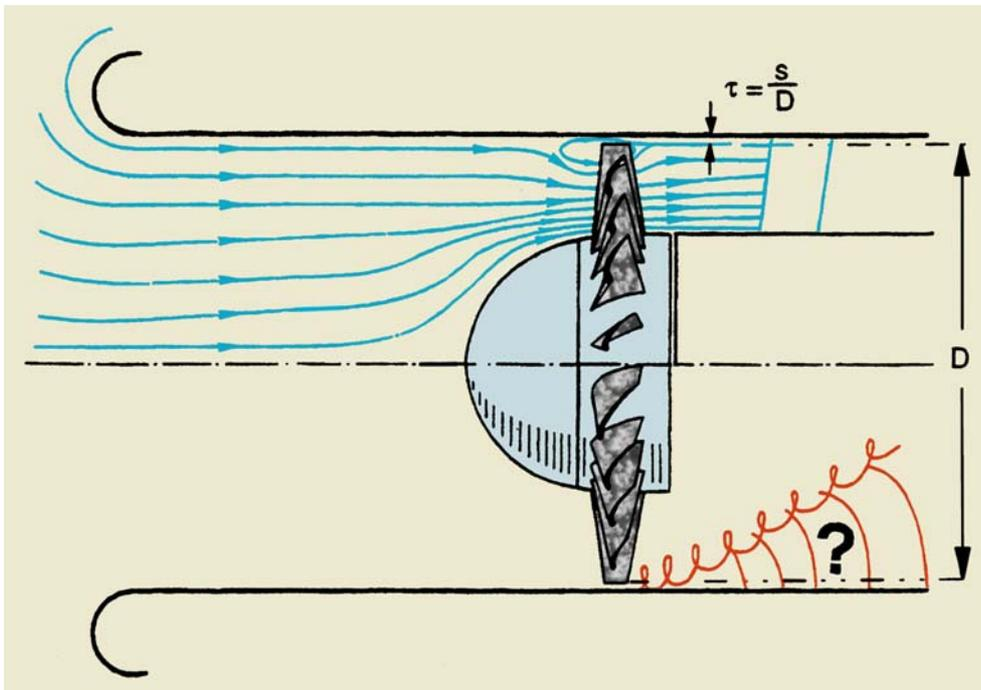
Fig. 1: Schematic flow diagram with generation of turbulence at the annular gap by difference in pressure
