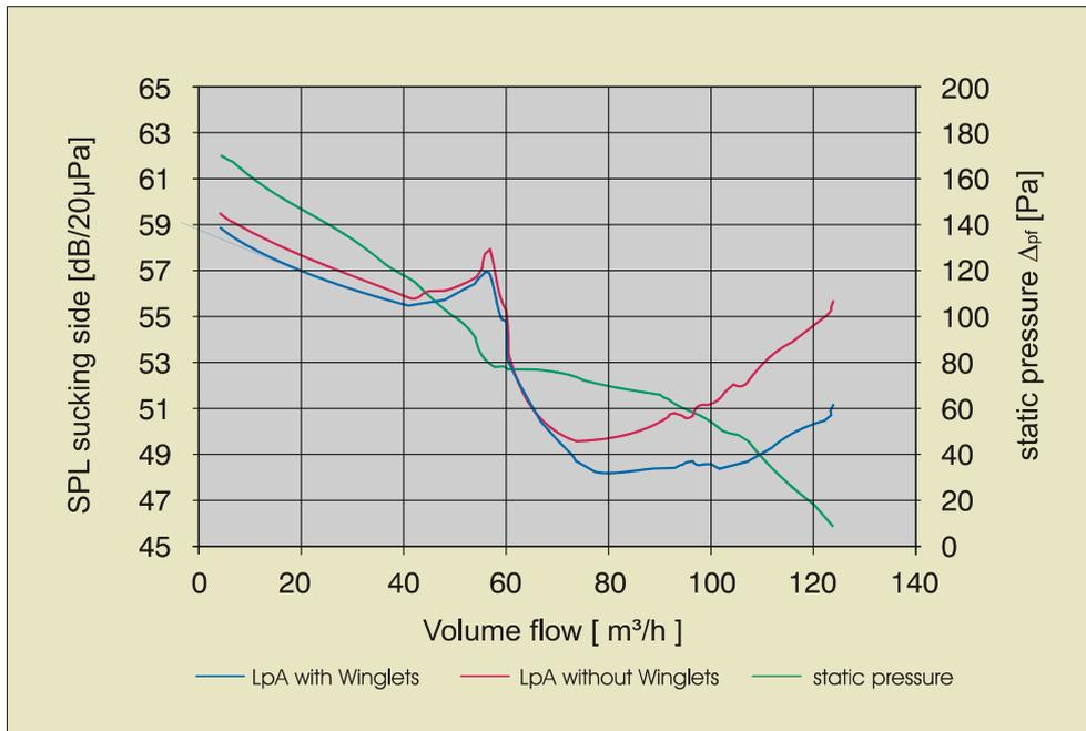
Fig. 3: Evidence that the winglets reduce the suction noise by up to 4 db(A)
