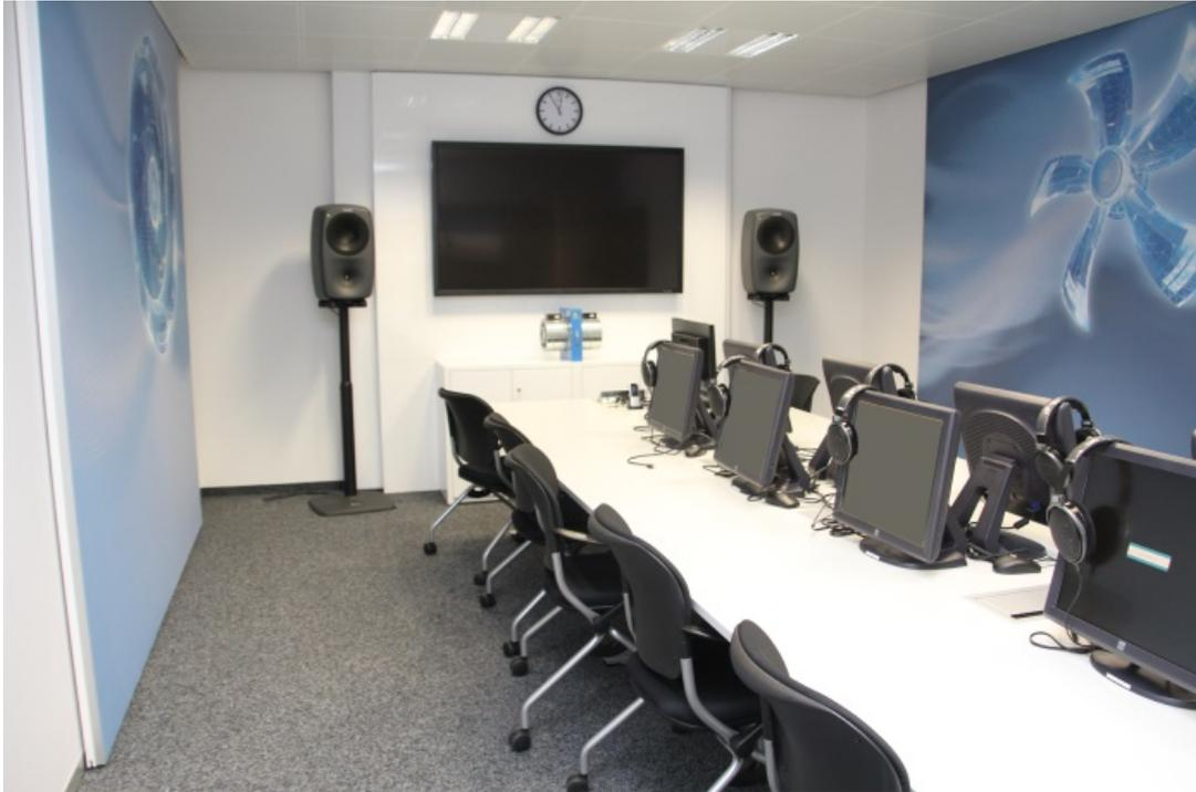
Figure 4: Searching for pleasant-sounding fans: This is a soundproof room with room for up to eight test subjects who listen to recorded fan sounds in various configurations. (Photo: ebm-papst)
