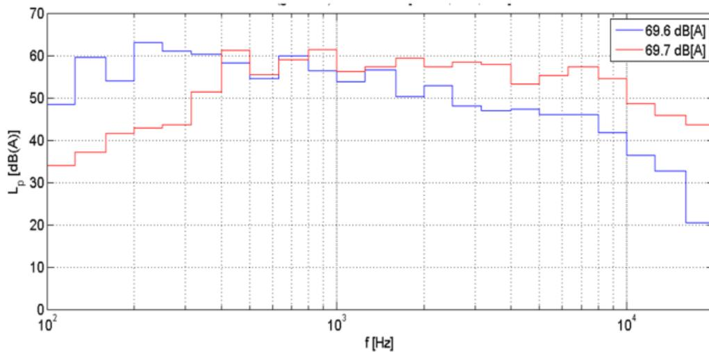
Figure 3: The noise spectra of a piece of music (blue) and a size 250 EC fan (red) are similar but are perceived quite differently. (Photo: ebm-papst)
