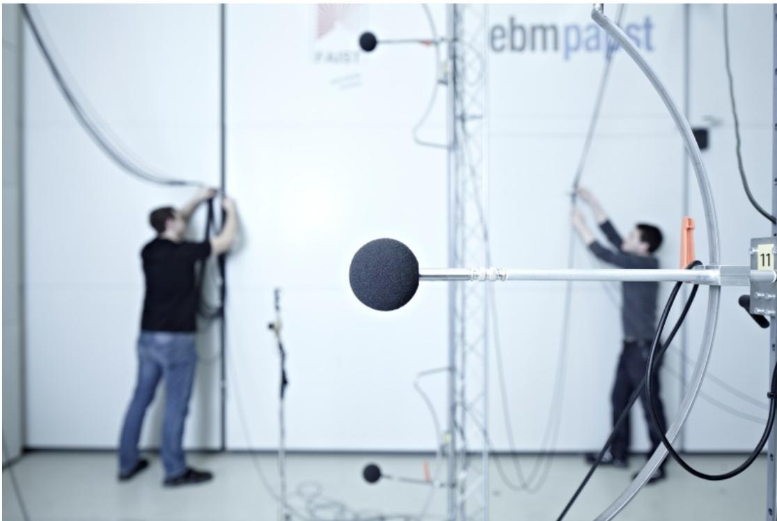
Figure 5: Specially positioned microphones for recording psychoacoustic parameters. (Photo: ebm-papst)
