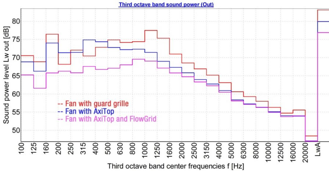
Figure 2: A noticeable reduction in noise can be achieved with the FlowGrid air inlet grille; it can be reduced even more in combination with the AxiTop diffuser. (Photo: ebm-papst)
