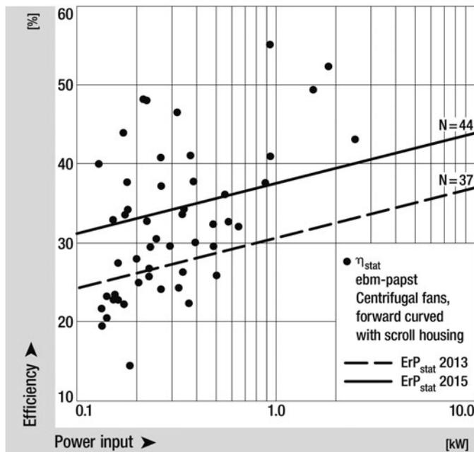
*Efficiency range for double inlet blowers: The black lines depict the limits as of 2013 and 2015. Not all fans are fit for the future requirements. It is also clear that for practically every fan that can no longer be used, already today there is an energy saving counterpart with GreenTech EC technology which does not just fulfil the directive, but significantly exceeds it.*
