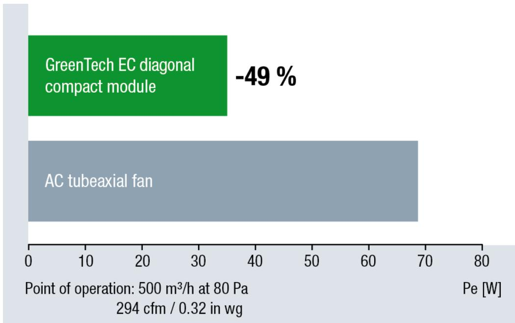
Fig. 4: Significantly lower energy consumption than an AC axial fan
