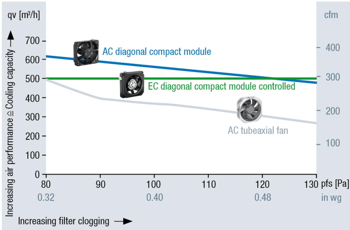
Fig. 3: Constant cooling capacity even as filter becomes clogged
