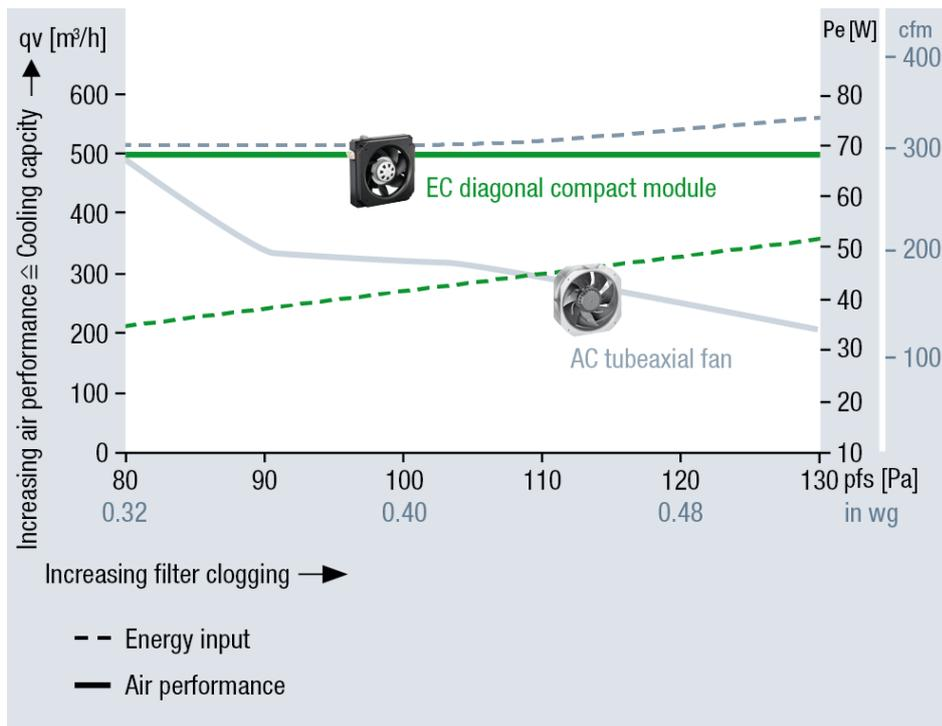
110 Fig. 5: The pressure-insensitive curve lengthens both the service life of the filter pads and the maintenance intervals.
