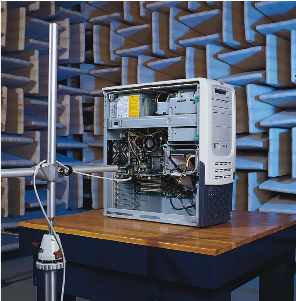
Fig 2: When used at the speed ranges that apply for cooling modern equipment, fans with Sintec compact bearings are audibly quieter than fans fitted with ball bearings
